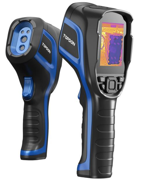
The TC004 is a handheld thermal camera that measures a wide range of temperatures, from -20°C to 350°C (-4°F to +662°F), and offers a 12-hour runtime. The high-resolution 256\*192 pixel infrared camera allows you to say goodbye to blurry images. The tool is ready for analysis with the standalone and the PC modes, enabling users to project and upload images from the TC to their PC.
