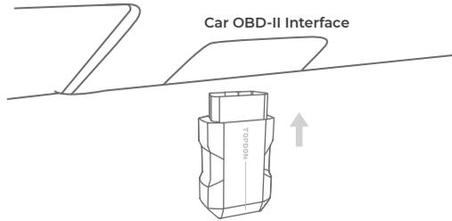
The vehicle's OBD-II port is usually located under the dashboard.
