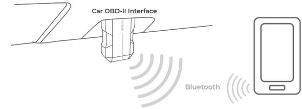
Tap **Vehicle Diagnosis** on the home screen, then tap **VCI** at the top right of the screen to establish a Bluetooth connection with the unit. When connection is established, the LED light on the unit will turn solid blue.
